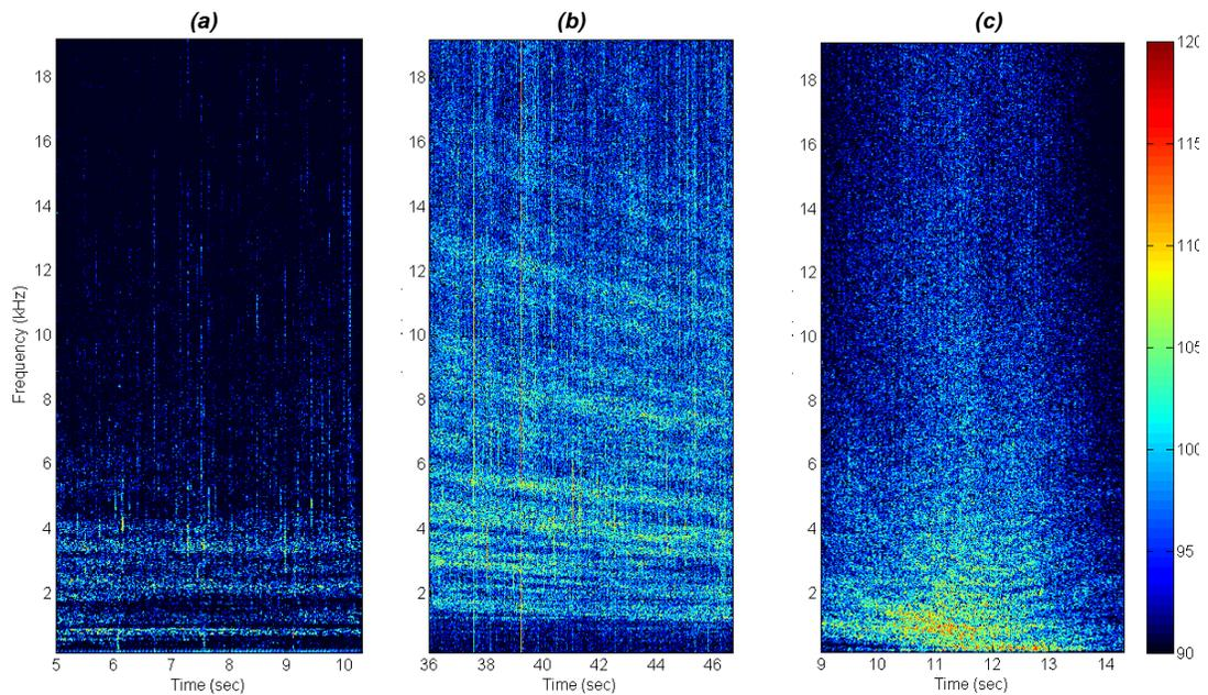
*Fig. 5. Examples of acoustic noise measurements for different kinds of surface vessels. Spectrogram representation (dB re. 1  $\mu$ Pa).*
