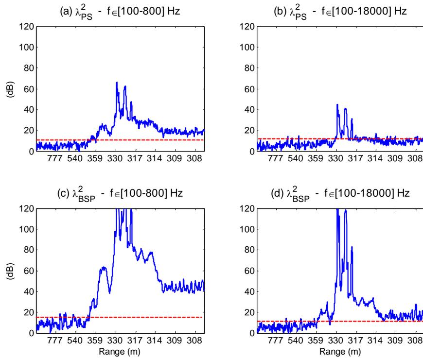
Fig. 7. Test variables detect a mid-sized vessel which approaches, manouvers and stops.
