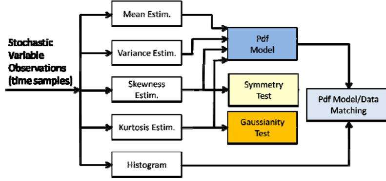
Fig.1. Block diagram of statistical analysis of acoustic noise observations.
