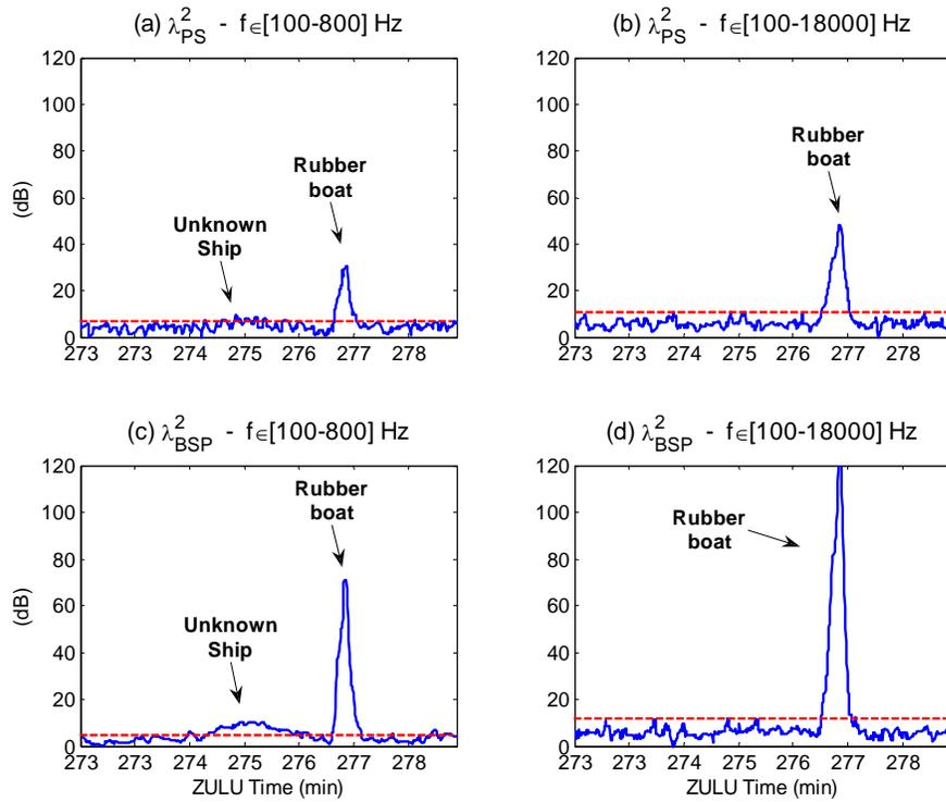
Fig. 6. Spectrum- (a)/(b) and bispectrum-based (c)/(d) test variables computed over two sub-bands while an unknown ship and a rubber boat pass in the area.
