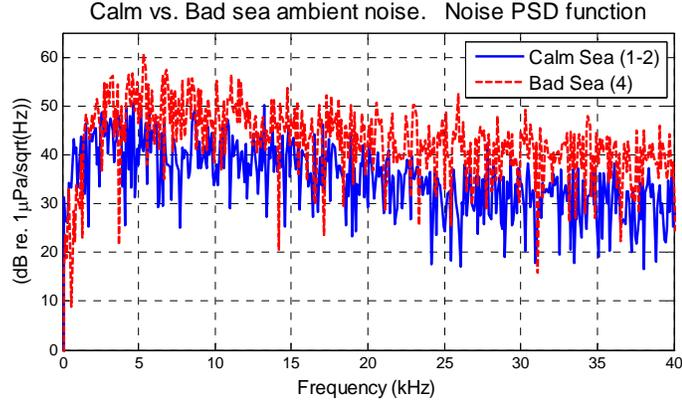
Fig.3. PSD functions of ambient noise computed over 2-sec-long datasets under different weather conditions (estimated sea state in brackets).
