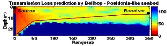
Fig. 8. Bellhop simulation when a noise source at 500 Hz is at the limit of the wedge.
