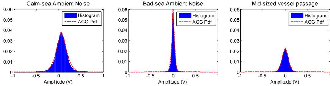
Fig. 4. Comparison of data histogram and pdf of the data sets analyzed in Table 1.
