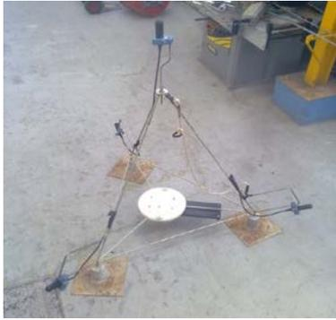
**Figure 6. Four-hydrophone volumetric array (tetrahedron) with electronics**
