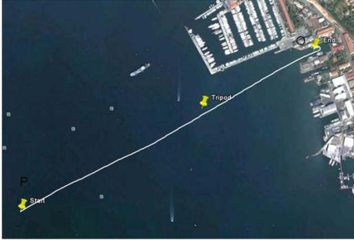
Figure 9. Google map of the experimental area, and the GPS track of the passage of an inflatable boat. The tripod location is outlined.
