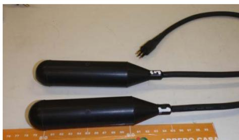
**Figure 4. Two of the preamplified analog hydrophones of a tetrahedron**
